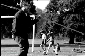
At left, Al Billups, civilian tech in charge, walking through a London park carrying a meter board (for leveling, to carry elevations from one point to another) while kids play soccer behind. Getting on Al's teams meant you were good at the work. Al got assigned some of the most sought after TDY jobs.
